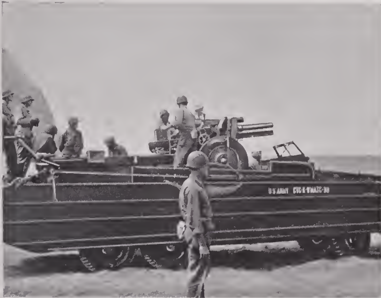
FIGURE 87. 105-mm howitzer can be handled easily by DUKW to fire on land.
